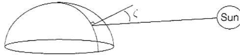
Figure 2.8. Illustration of the solar zenith angle ( \zeta ), defined as the angle between the direction of a direct beam of radiation from the sun and a line normal to the surface of the Earth.
