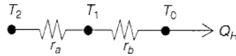
Figure 2.15. Illustration of three different temperatures ( T_2 > T_1 > T_0 ), separated by air with resistances r_a and r_b , and with flux Q_H .
