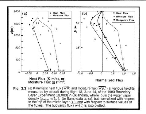
ML can increase substantially during that time interval. To remove these effects, micrometeorologist often normalize their plots. Height is normalized by dividing by the depth of the ML,  $z_i$ . Flux is normalized by the concurrent surface value of flux observed (or estimated).
