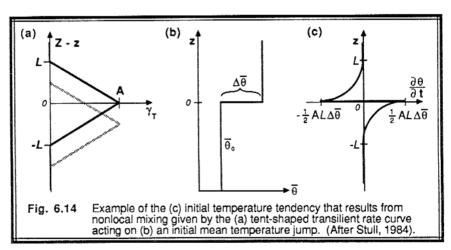
**Solution:** The transilient rate curve indicates that the largest eddies (i.e., large values of |Z-z|) present for this case are of size L. Thus, for z < -L and z > L, mixing can not change the temperature because the smaller eddies (less than L) are mixing air of the same temperature. Air of different temperature from the other side of the temperature jump is out of reach of these small eddies. Thus, by inspection we can write the first part of our answer:
